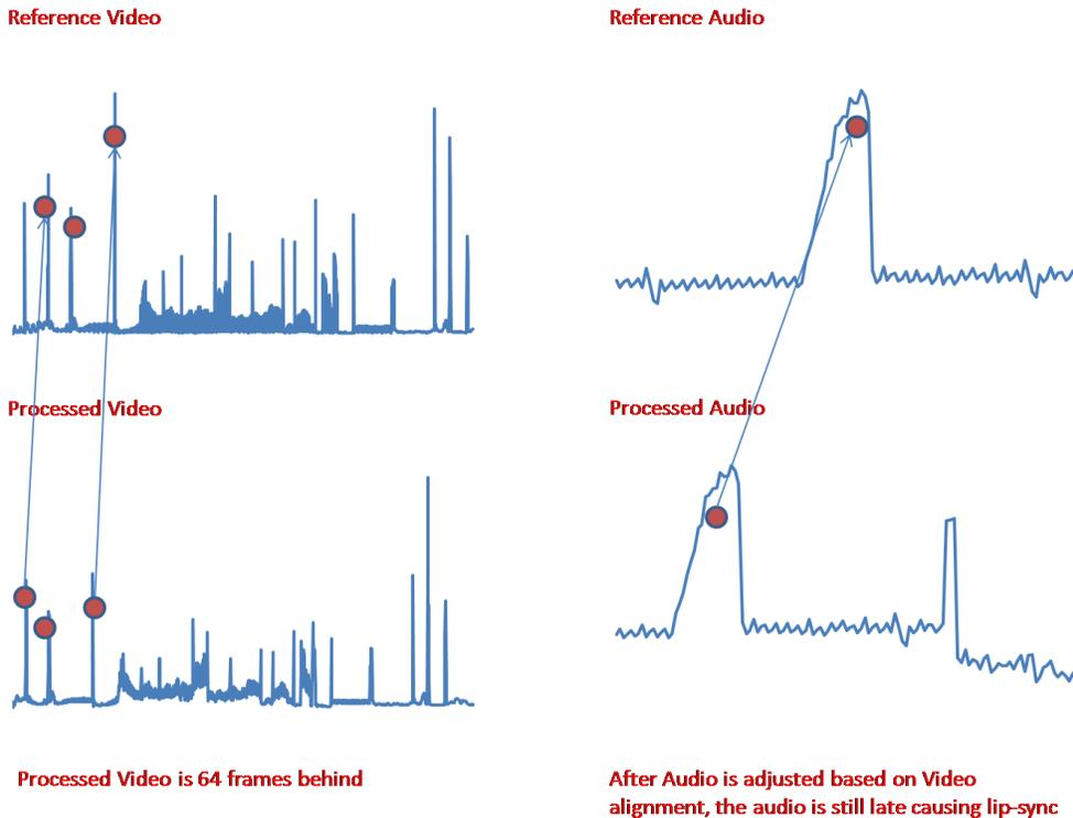
The reference and processed audio and video are analyzed separately, and an offset for each is calculated. This offset is the delay caused by processing. In theory the audio and video delay should be equal. If they are not, then the difference could create a lip-sync problem.
