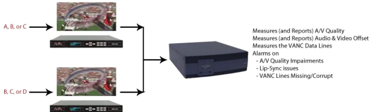
RTM takes 2 SDI feeds, professional adapters are available for component, HDMI, etc., and it aligns the video and the audio.
