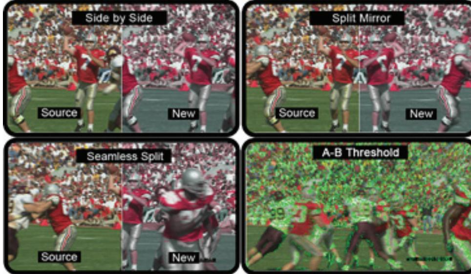
To simplify the work flow, any video sequence can be played while capturing another video sequence, thus, combining the video server, capture device, viewer and video analyzer into one unit. By doing this ClearView controls the test environment, which allows for automated, repeatable, quantitative video quality measurements.
