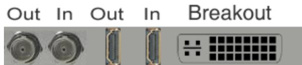
The CV-SDI-IO-LHi module on ClearView Shuttle and QA models records and plays HD/SD video and audio. It is capable of up to 1080P/60Hz record and/or playback. ClearView stores the video data as 100% uncompressed 8/10-bit 4:2:2 Y'CbCr. The inputs and outputs are any of HDMI, HD-SDI and Component, Composite, S-Video along with digital and analog audio.
