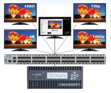
The Venue Recorder application provides the ability to record multiple uncompressed video signals and multiple resolutions of video, audio, and ancillary data. Targeted for use with Venue Player or ClearView Analyzer systems when more than two sources need to be recorded, the Venue Recorder allows incoming content channels to be independent of system playback functions.
