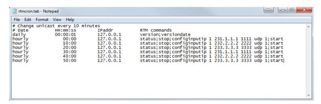
In this example the scheduler is telling RTM to switch unicast addresses every 10 minutes. A series of commands is separated by semicolons to check the status, stop RTM, configure the new input, then start back up again.
