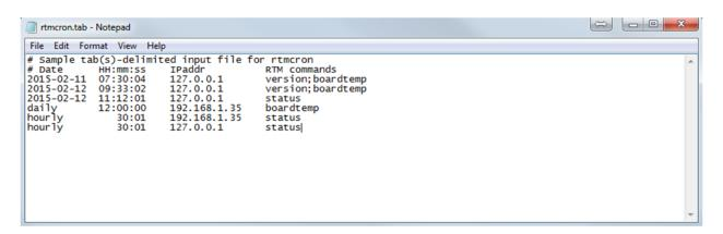
In this example, three sets of commands will be sent at a specific date, and time. One command to check board temperature will be sent daily, and the status of two RTM's will be checked hourly.
