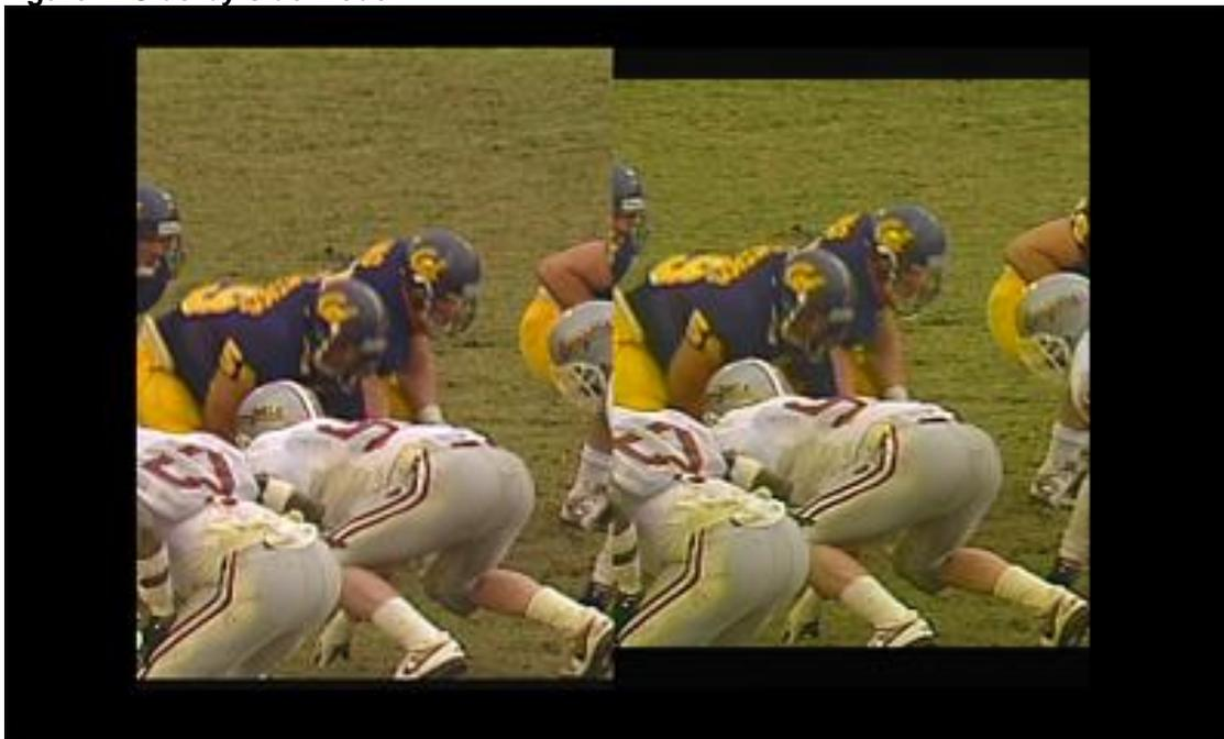
As a first step, a window will be drawn around both video sequences to crop the original video sequence. To get the box exactly right, the pixval tool will be used to find the first occurrence of non-black at the top and the first occurrence of black at the bottom of the video sequence on the right. With these Y offsets measured, a window can be drawn using the window command.
