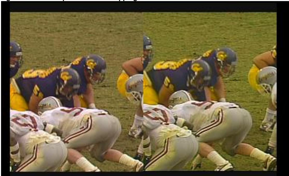
At this point the video sequences are now the same size, but they are not aligned. Using ClearView's spatial alignment, the video sequences were found to be off by  $x=-6$ ,  $y=-16$  (the video sequence on the right is higher and further to the left).
